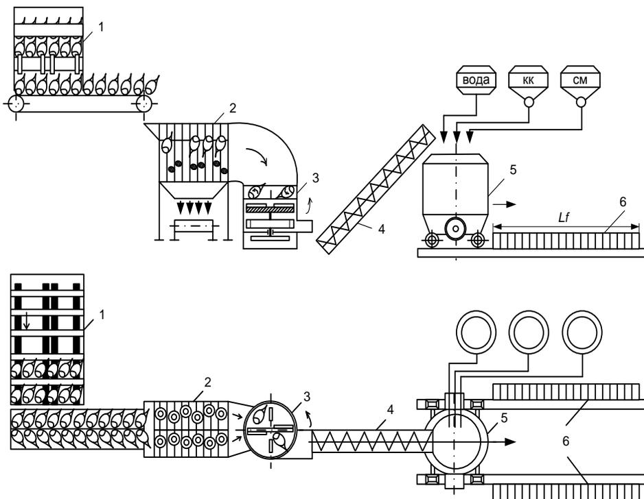
Figure 3: Structurally-technological scheme of line preparation and distribution of feed mixtures for pigs
