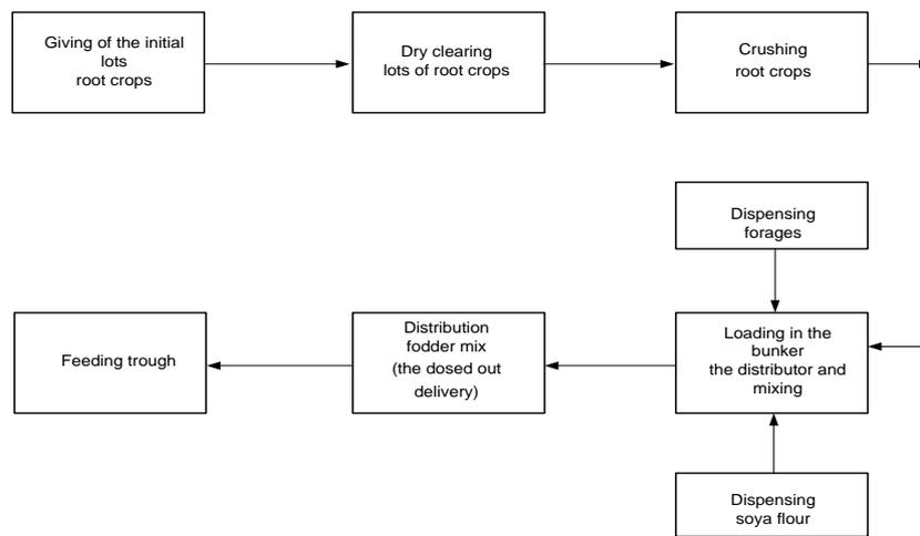
Figure 2: Block diagram of the process of preparation and distribution of feed mixtures for pigs
